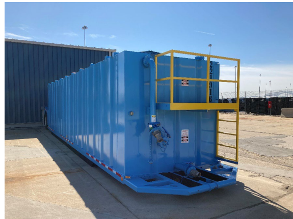
Figure 2 Frac Tank for water management at DMT
