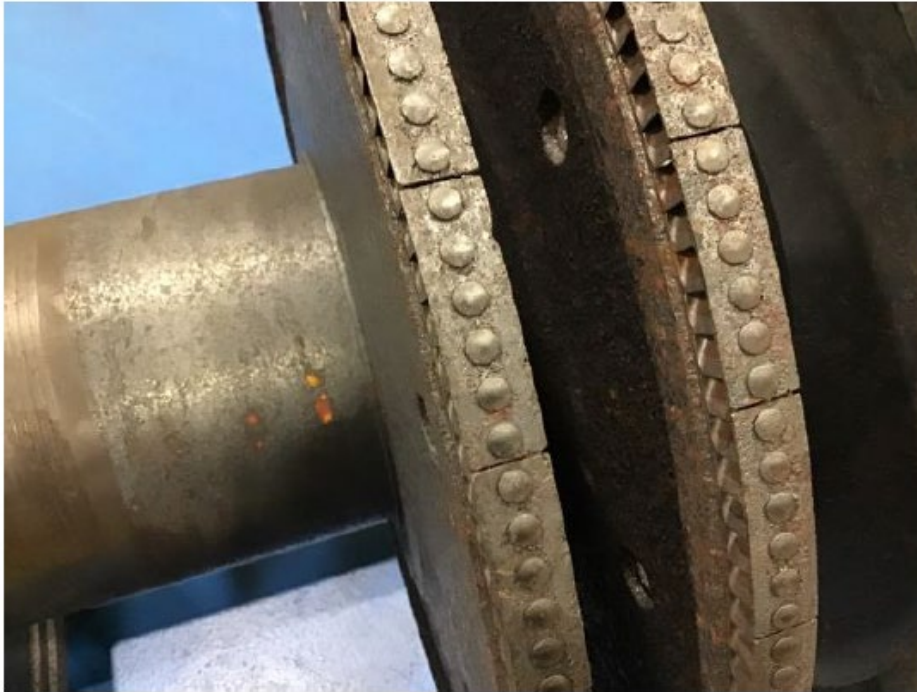
Description: as-received rotor depicting damage to shaft, wheel, blades and shrouds.
