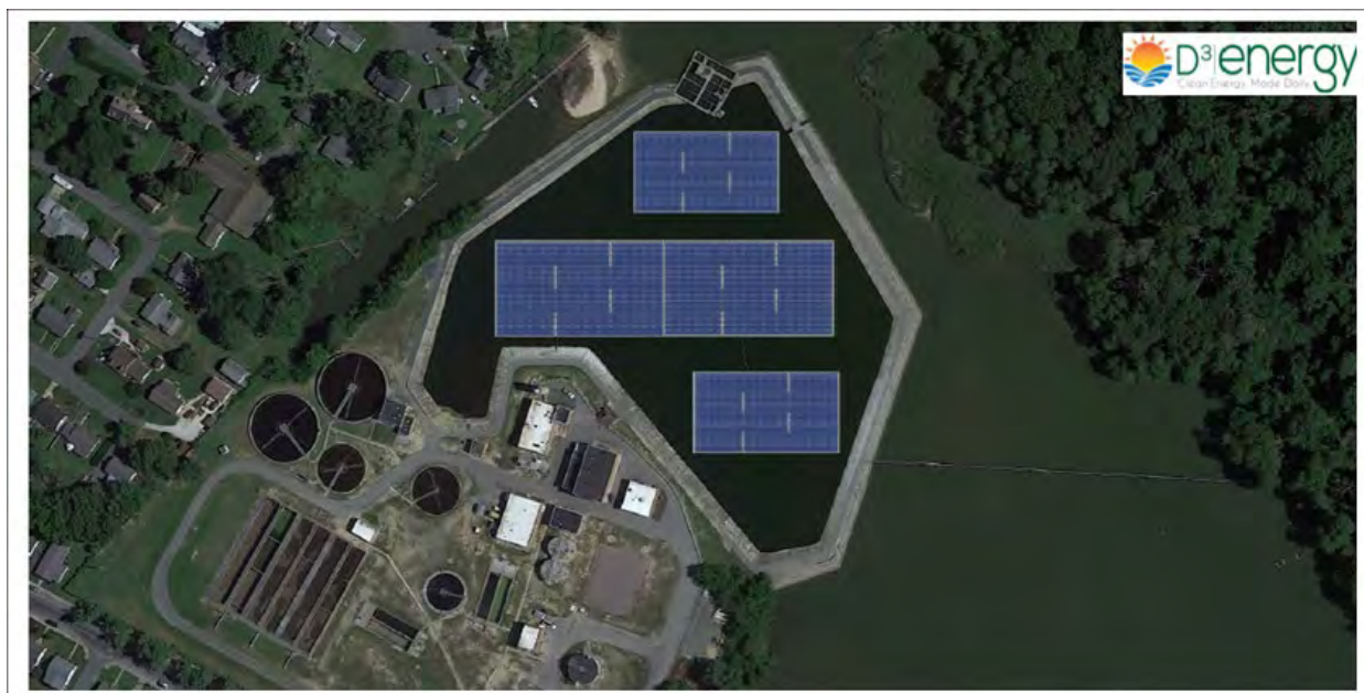
Figure 14 – Proposed Floating Photovoltaic (PV) Cells at the City of Cambridge WWT Shellfish Protection Pond (courtesy of D 3 Energy, LLC)
